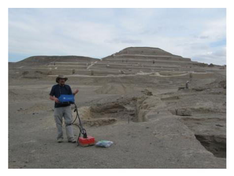
Fig. 14.6 Georadar system
