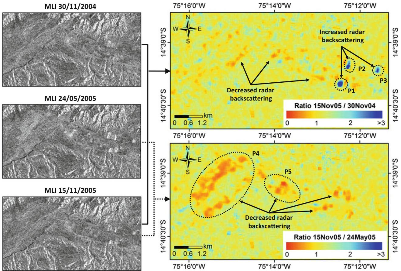
**Fig. 3** Amplitude change detection maps obtained over the Rio Ingenio floodplain by ratioing the backscattering coefficient ( $R\sigma^0$ ) estimated in November 2004 and November 2005 (yearly basis), and
