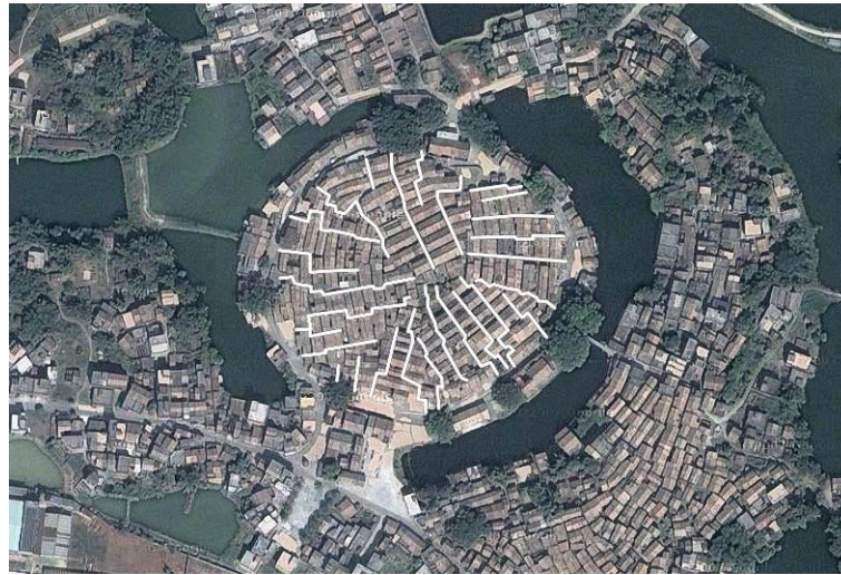
Fig.7 Schematic diagram of longitudinal drainage system in Xiangang Village (Drew by the author with reference to Google Map)
