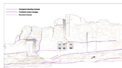
Fig.4. South elevation: Three types of fractures are evident; an old geological one (violet), a post excavation (blue), a structural one (red).
