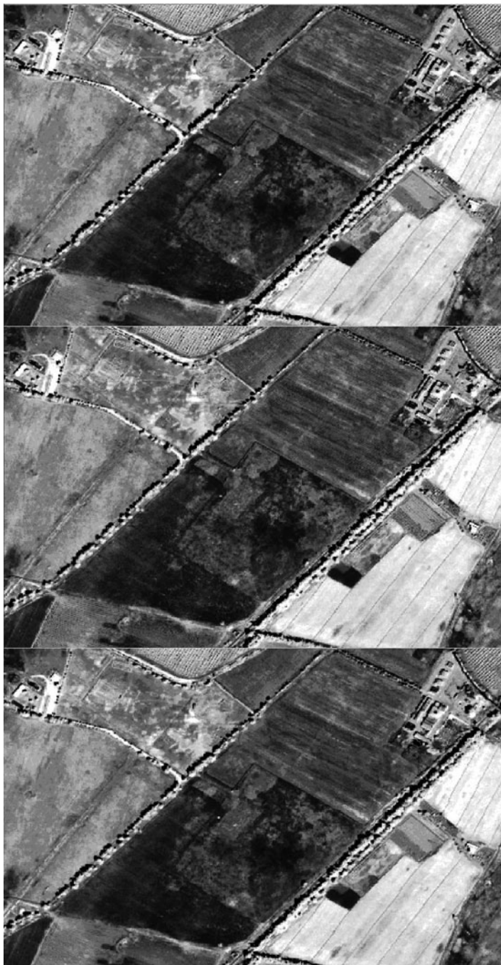
Fig. 4.10 Visualization of NIR pan-sharpened images obtained by using Gram Schmidt ( upper ), PCA ( medium ) and Wavelet transform ( lower ) methods
